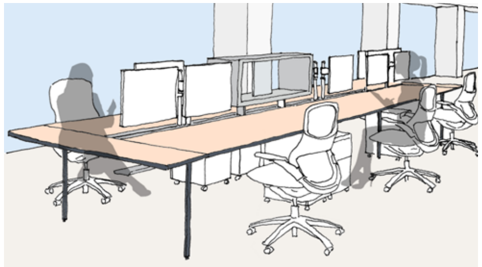
Figure 3: Benching configurations allow efficient shared access to power and communications distribution, temporary tightening of individual workspaces, and future expandability.
